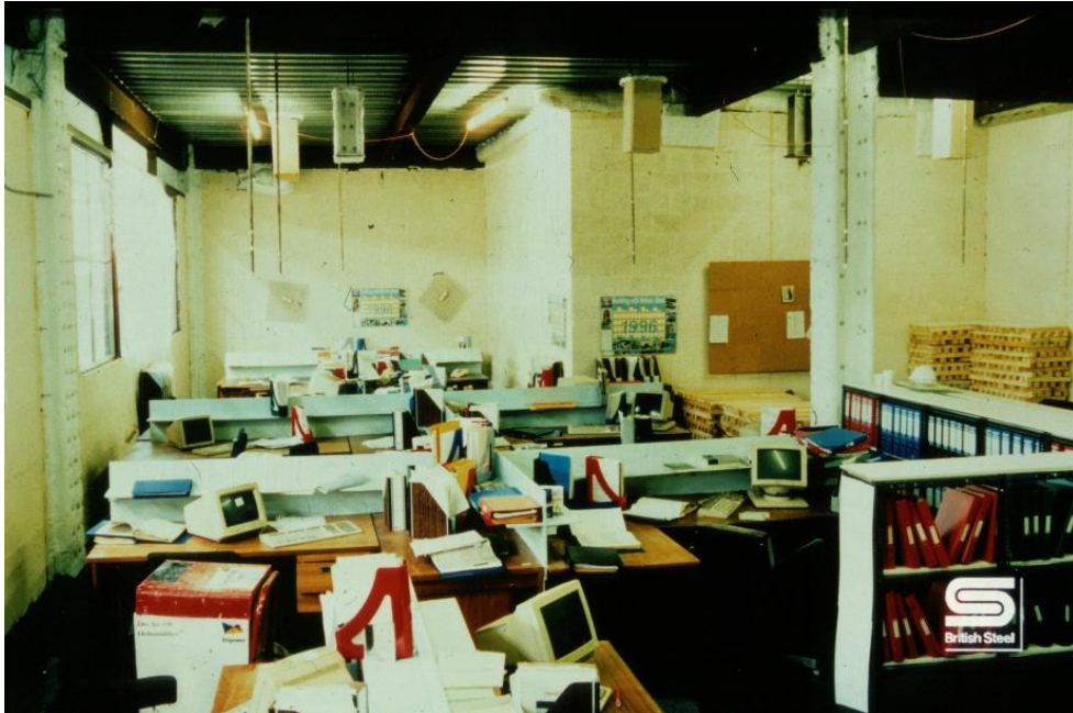
Fire Load with Real Office Supplies (500 MJ/m 2 )
