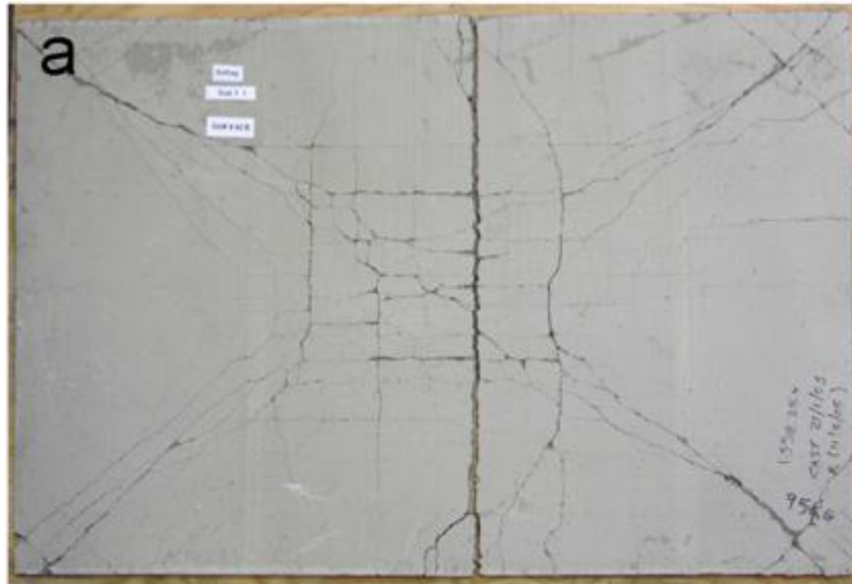
Failure by tension in the reinforcement
